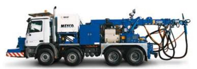
Totally mobile spraying system with all necessary components on roadworthy carrier vehicle. Power take-off enables operation with or without site power supply ensuring absolute flexibility. MEYCO Maxima, a specially developed manipulator with huge spraying range but can be extended in small tunnels.
