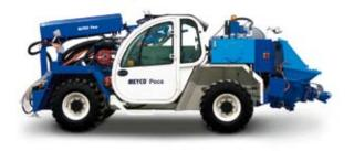
Extremely compact, very mobile spraying unit designed for smaller tunnel profiles and incorporating basic MEYCO technology. MEYCO Rama spraying manipulator, MEYCO concrete pump, peristaltic dosing pump mounted on a rigid 4WD, 4WS chassis.
