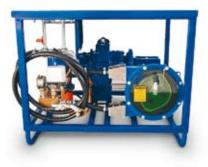
Dosing unit for liquid admixtures for any sprayed concrete applications. Peristaltic hose pump mounted within steel frame and cover. Volume of additive is set with hand wheel on variable drive. The amount supplied is visible on flow indicator display.
