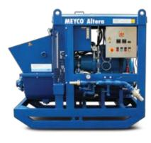
A twin-piston pump suitable for concrete conveying, hand-spraying, grouting, repair work and spraying with small manipulators. Extremely simple in construction and operation but still maintains CE standards of safety. It is very compact, durable and versatile enough for any site in the world.
